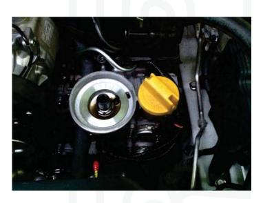
2. Assemble the large 'O' ring to mounting face. Assemble the 'O' ring supplied with the dash fittings to the dash fittings, now assemble the dash fittings to the adaptor using some engine oil to lubricate the 'O' rings.
