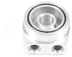
3. Install the sandwich plate on top of the riser plate having smeared some oil on the 'O' ring. Fit and screw the retaining socket to align and hold the two in place. Tighten to 30 Nm torque.
