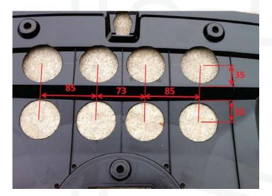
13. Refit the lower under tray to underside of the vehicle. (Note the front 3 centre scrivetts can no longer be used as the engine oil cooler is located in the mounting hole area).
